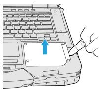
$3. \quad \text{Insert an option until it securely fits the connector}.$
