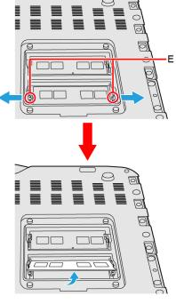
3. Carefully remove the RAM module from the slot.
