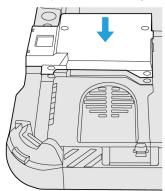
Tighten the screws (C) firmly.
